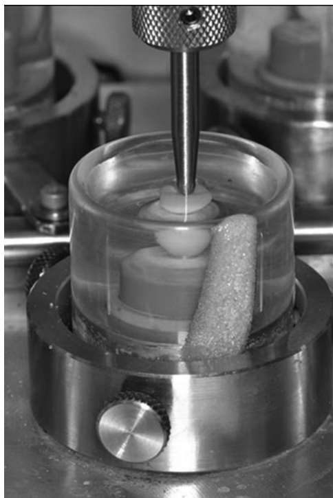
Figure 1 Apparatus for mechanical cycling. The loading device was positioned on the center of the occlusal surface.
